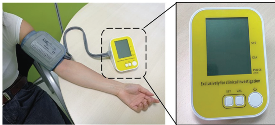
Figure 1 Remote ischaemic conditioning device. The remote ischaemic conditioning device is very similar to a blood pressure monitor, but with modification to maintain a target pressure of 200 mmHg for 5 min, causing ischaemia in the upper limb. In remote ischaemic conditioning, brief, reversible episodes of ischaemia followed by reperfusion in one body part (usually an arm) render remote tissues and organs resistant to injury.
